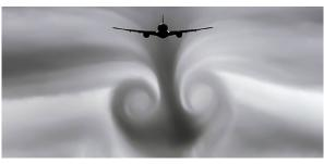
▲ FIGURE 15 On the left, a modern plane winglet. © PierreSelim, CC BY-SA 3.0 On the right, wingtip vortices in the wake of a plane without winglets. © Steve Morris
